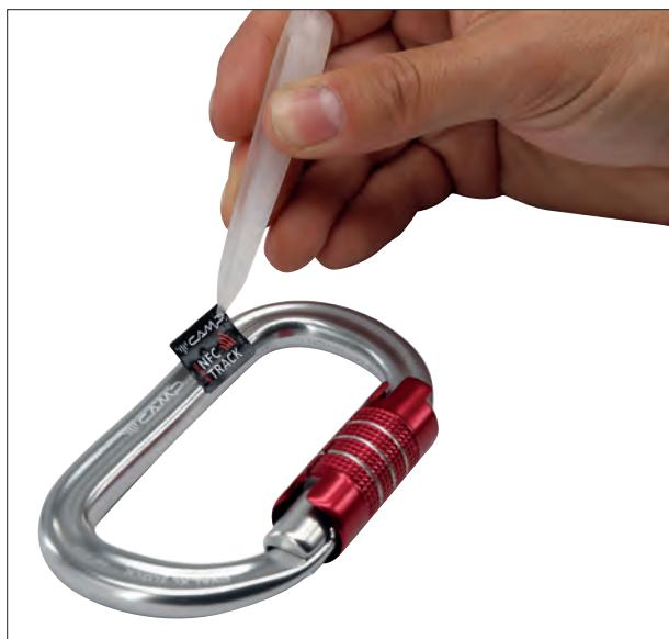
Adhesive chip, designed for metal products, for the individual identification, control management and PPE allocation. Digital traceability is made possible by the HF RFID technology, which allows for immediate reading with any smartphone that is equipped with NFC functionality and professional use with the C.A.M.P. NFC TRACK universal reader (ref.3251).
